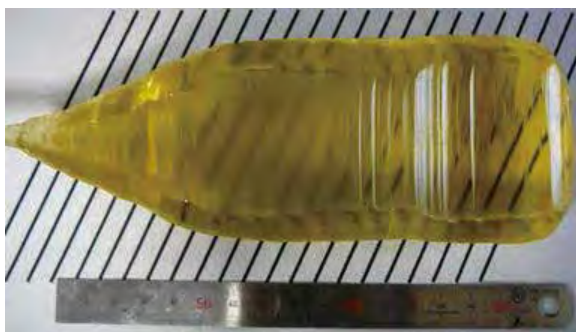
Fig.1 Novel langasite-type single crystal.
